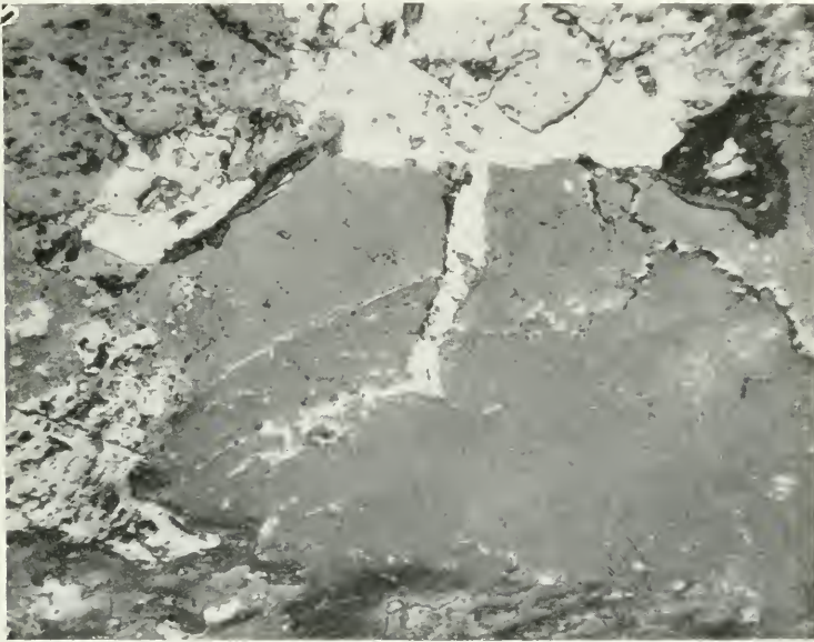
Fig. 23—Polished surface of ore, showing veinlets of sulphides (white) replacing or impregnating rock; magnified 88 diameters; Creighton mine, Sudbury area, Ontario. The sulphides replace or impregnate all the rocks at Creighton mine, whether they consist of norite, granite or greenstone. Photomicrograph by Wm. Campbell.
